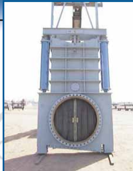
54" Rolling Slide Gate Valve for blower inlet isolation 7.6 PSIG @ 600°F
