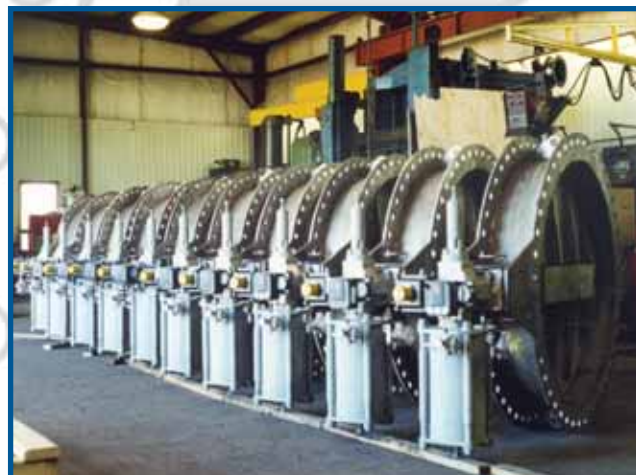
48" Pneumatically Operated Tadpole Butterfly
