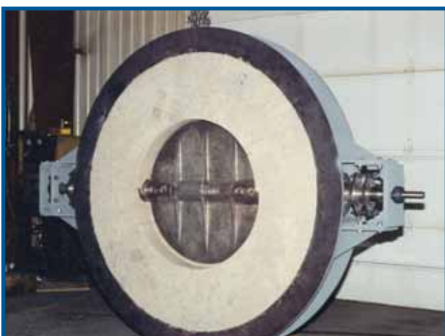
66" X 36" Refractory Lined Butterfly Valve
